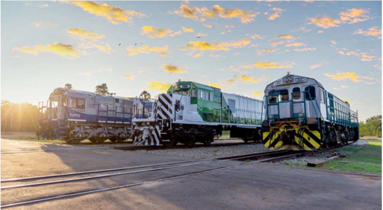
*Progress Rail EMD® GT38H hybrid, SD40JR Joule battery-electric, and GT38JC Joule. Progress Rail photo*
