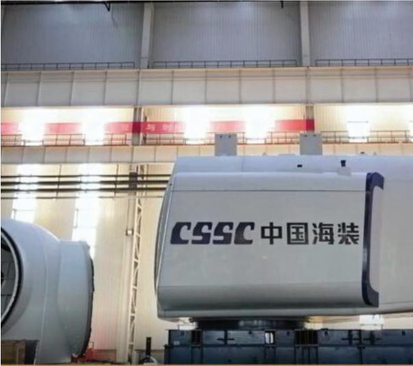
*The rotor hub and nacelle of a new 18-MW offshore wind turbine from a subsidiary of China State Shipbuilding Corp. is shown at its factory. Source: CSSC Haizhuang*
